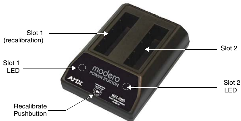
FIG. 32 Component locations on the NXT-CHG
